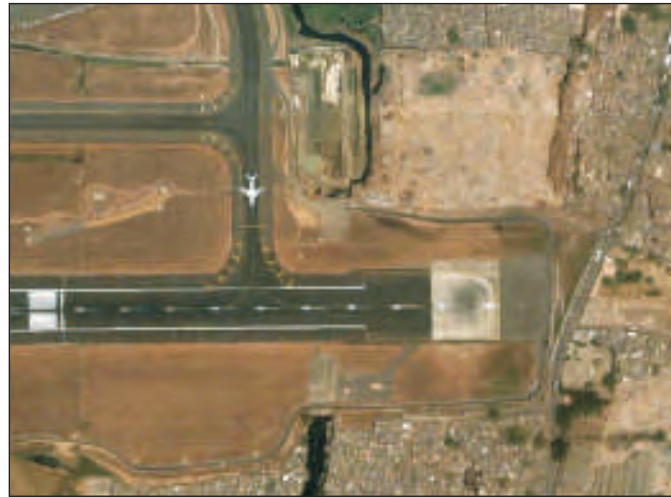
Figure 3.7- Temporary diversion of Mithi River's course for construction of a box culvert under proposed taxi-bay extension (April 2005) Photo Courtesy: Google Earth Imagery
