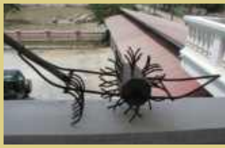
Photo 8.11 Simple weeder designed by Nong Sovann (Cambodia) with wooden axle, large nails, rake, and metal rods, costing less than USD 3.
