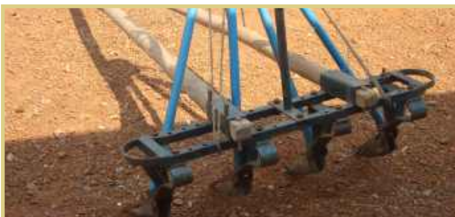
Photo 3.6 Four-row seed drill for rainfed SRI
