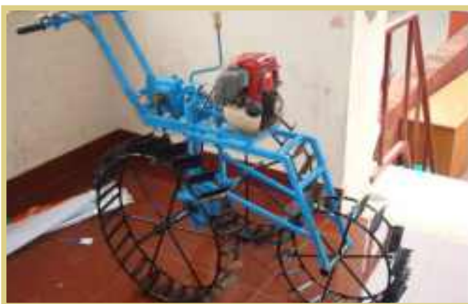
Photo 8.19 Three-row motorized weeder (TNAU)
