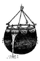
For a 300 arms length deep well, the moment the *charas* is filled up, the first pair of oxen covers 150 hands on the sloping *saran*, bringing the *charas* halfway. The string is then skilfully tied to the second pair in the twinkling of an eye, after it is removed from the first pair, which is guided up while the other pair continues to draw the *charas* for the remaining distance. The gurgling *charas* is emptied; thus the underground water starts flowing to the surface of the earth.
