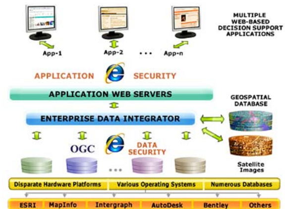
Diagram: 15- Process flow of GIS & MIS based database creation
