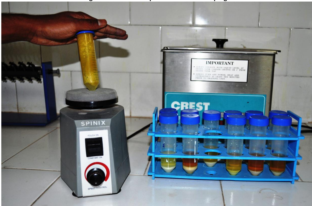
Figure 5. Extraction of pesticide residues - in progress
