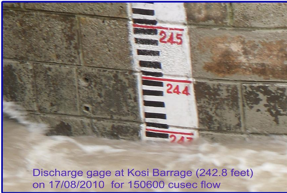
Photo 1. The River Kosi Discharge Gage Reading at Bhimnagar Barrage on 17.08 2010 at 1200 Hrs.
