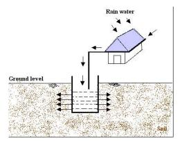
As a result of backwashing, a fresh water zone is created around the backwashed well. So the water in the well is assured to be clear and safe all the year The physical and chemical properties of water become more acceptable.
