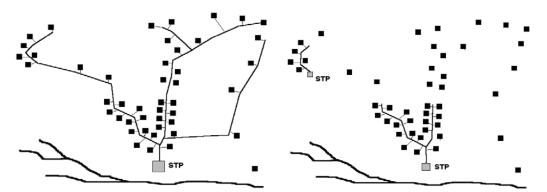
Figure 3. Concept of Centralized vs Decentralized Sewerage Layouts
