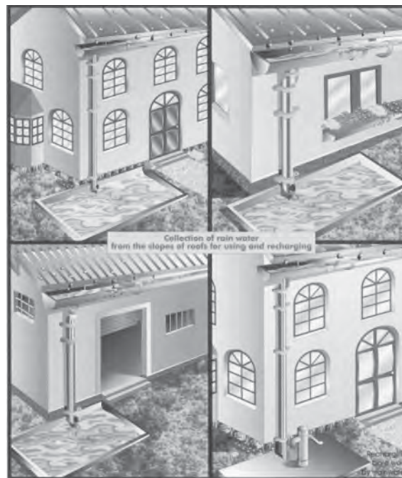
Fig. 10.9 Rooftop Rainwater Harvesting
