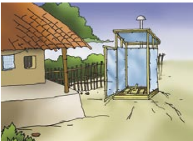
Figure-38, Superstructure-plastic made
