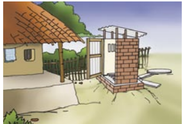
Figure-37, Superstructure-brick made
