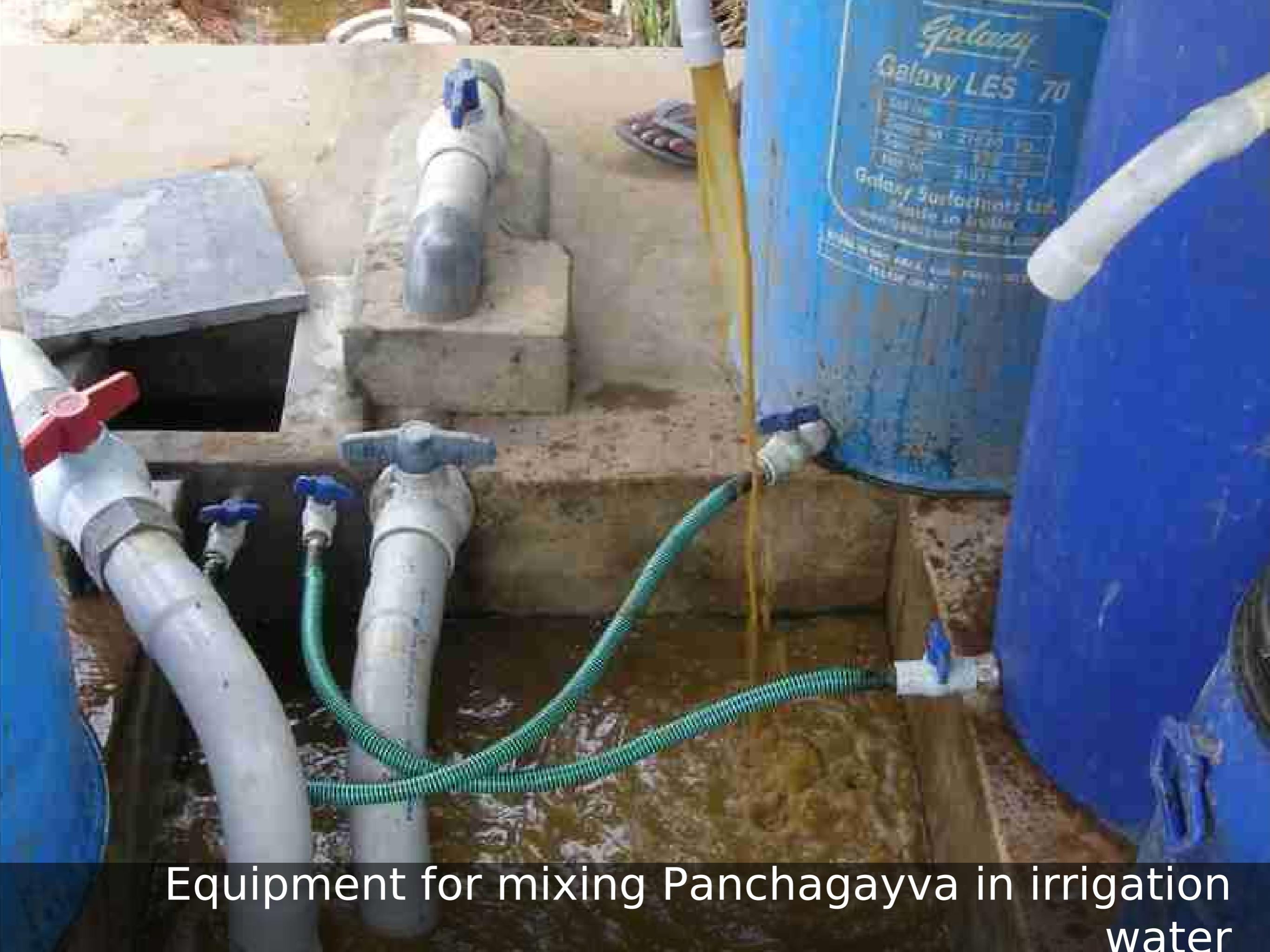
Equipment for mixing Panchagayva in irrigation water
