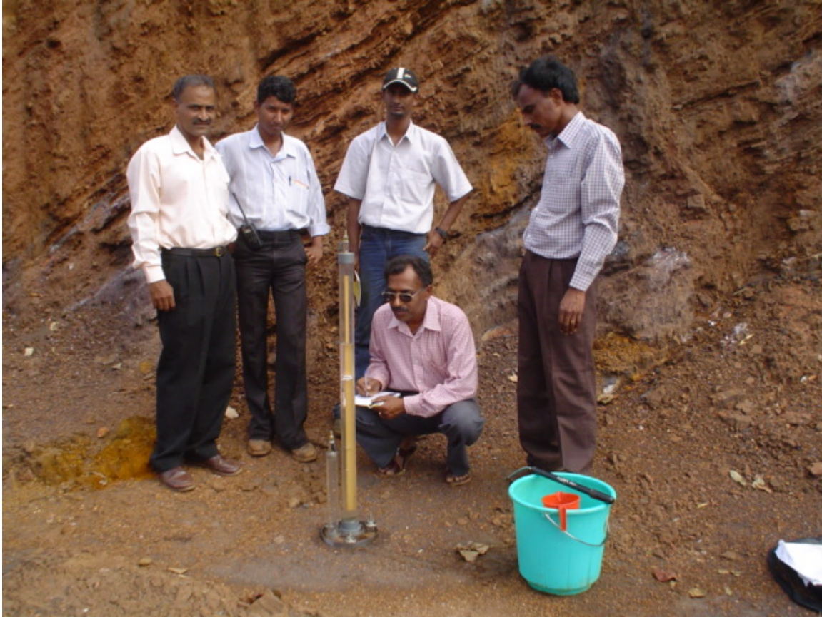
Figure 10: Measurement of Hydraulic Conductivity in Laterite Soil
