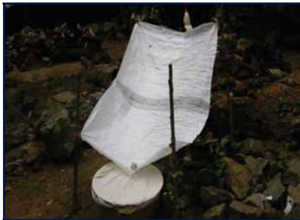
Simple form of Rainwater Harvesting
