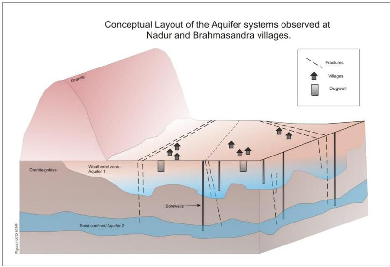
Figure 3: Conceptual layout of the Aquifer Systems observed at Nadur and Brahmasandra villages
