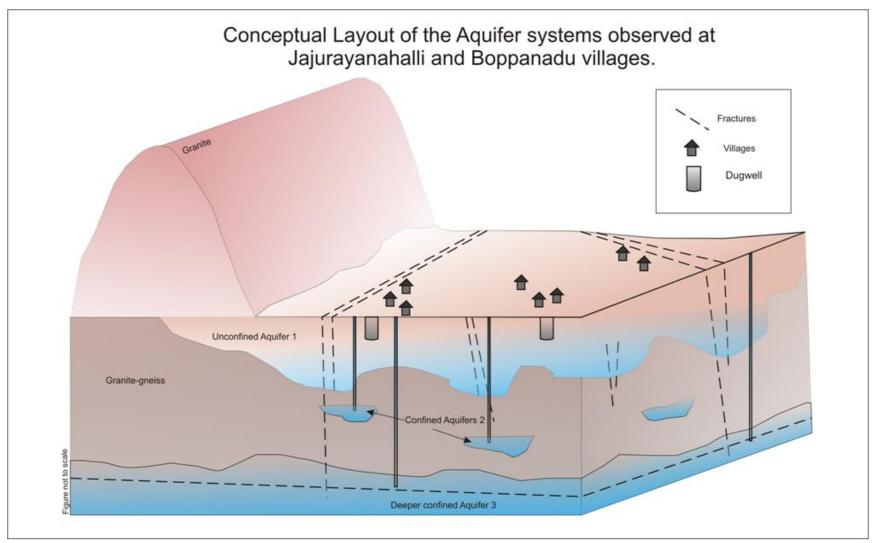
Figure 2: Conceptual layout of the Aquifer Systems observed at Jajurayanahalli and Boppanadu villages
