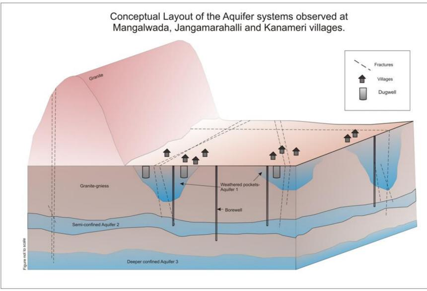
Figure 1: Conceptual layout of the Aquifer Systems observed at Mangalwada, Jangamarahalli and Kanameri villages
