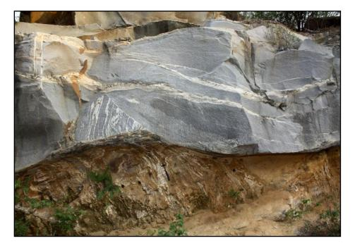
**Photo 5:** Incipient weathering – fresh granite overlying weathered granite.
