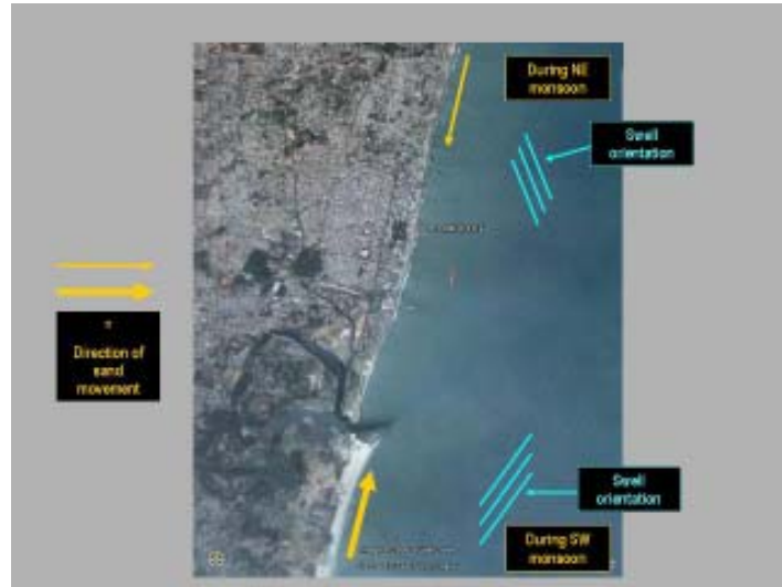
Figure 3 & 4: Mechanism of sand transportation along the east coast of India
