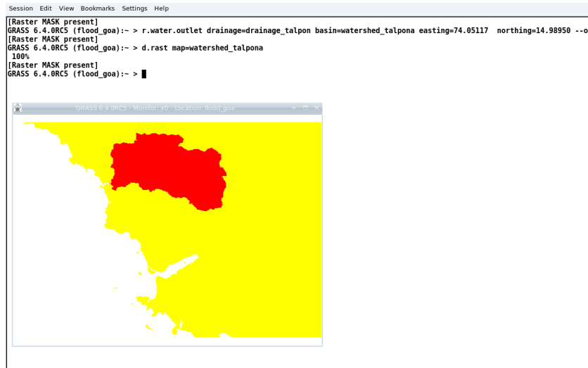
Figure 21: Creating watershed area over the selected location. The area plotted in red is the watershed area over the selected location.
