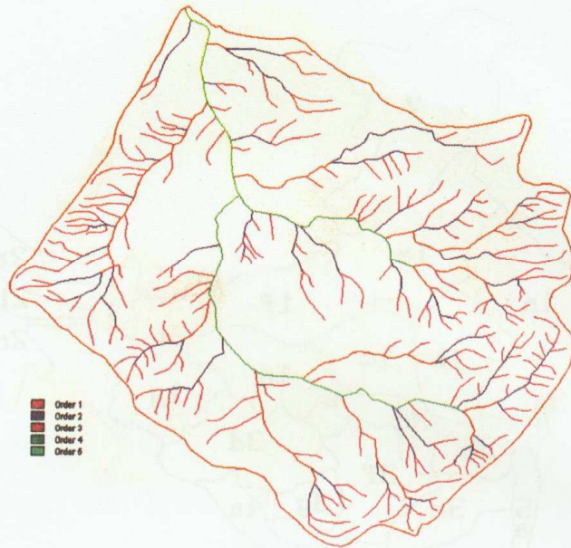
Fig. 2 Drainage network map of the bridge catchment no. 527
