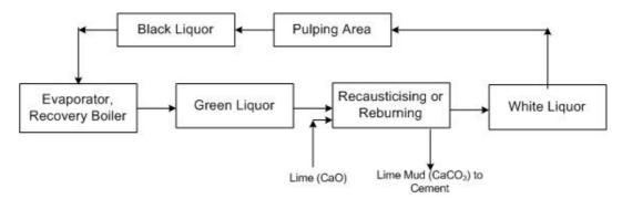
Figure 3-5: Schematic Diagram of Chemical Recovery Flow Process
