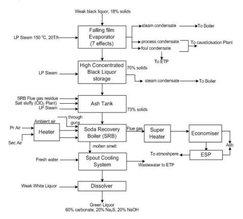
Figure 3-6: Soda Recovery Process
