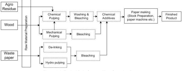
Figure 3-1: Typical Pulp & paper Manufacturing Process
