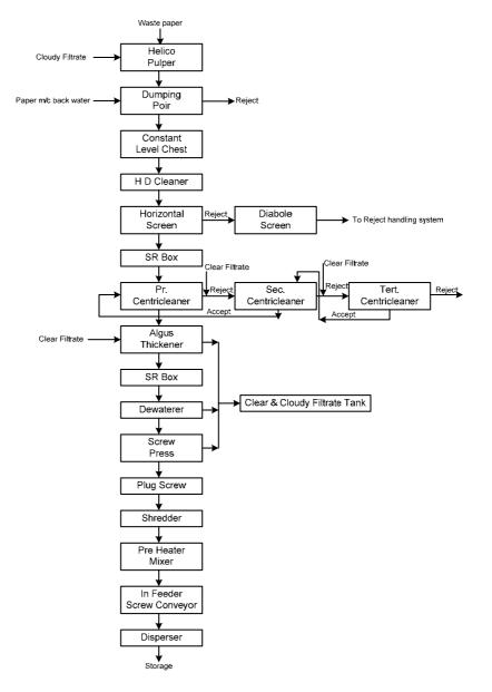
Figure 3-4: Secondary Fibre or Wastepaper based Manufacturing Process
