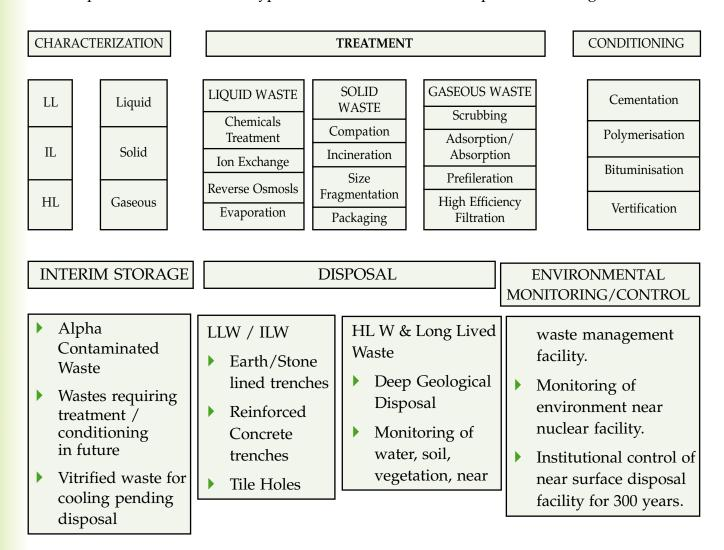
Fig. 5.4 Management Methodology of Different Types of Radioactive Waste
