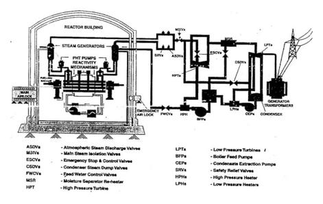
Fig.5.1 Pressurized Heavy Water Reactor (PHWR)
