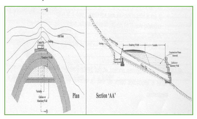
Figure 5.1: Schematic Layout of Waste Management in case of Hilly Areas (Source: Environmental Codes of Practices, 2004 – Ministry of Rural Development, Gol)
