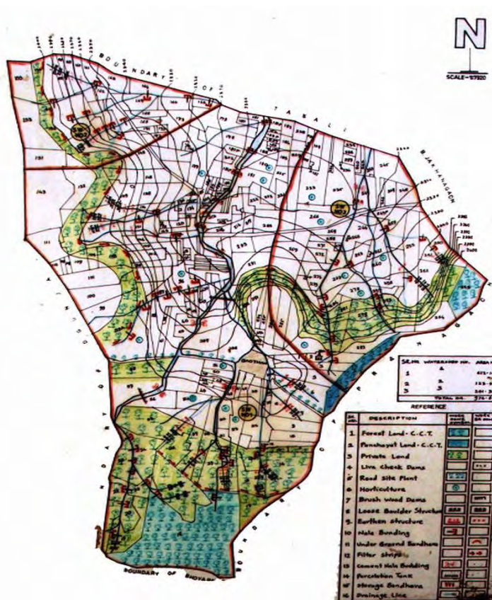
Figure.32 Location of soil and water conservation structures constructed.
