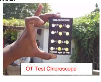
chlorine testing is essential, after taking a sample. The two methods are the Orthotolidene Test) and the DPD Tablet method. on colour intensity using a simple To overcome the problems of water quality in system storage, cleaning, proper mixing and
