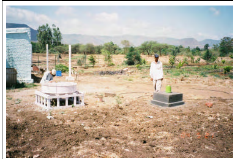
Evaporimeter and rain gauge installed at Chale
