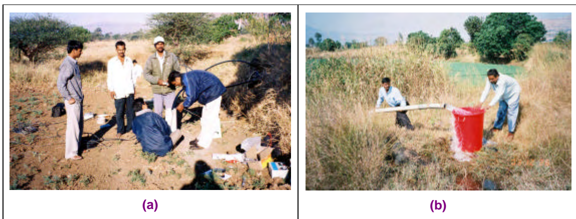
Pumping tests conducted on boreholes involved measurement of water levels (a) and measurement of discharged water (b)
