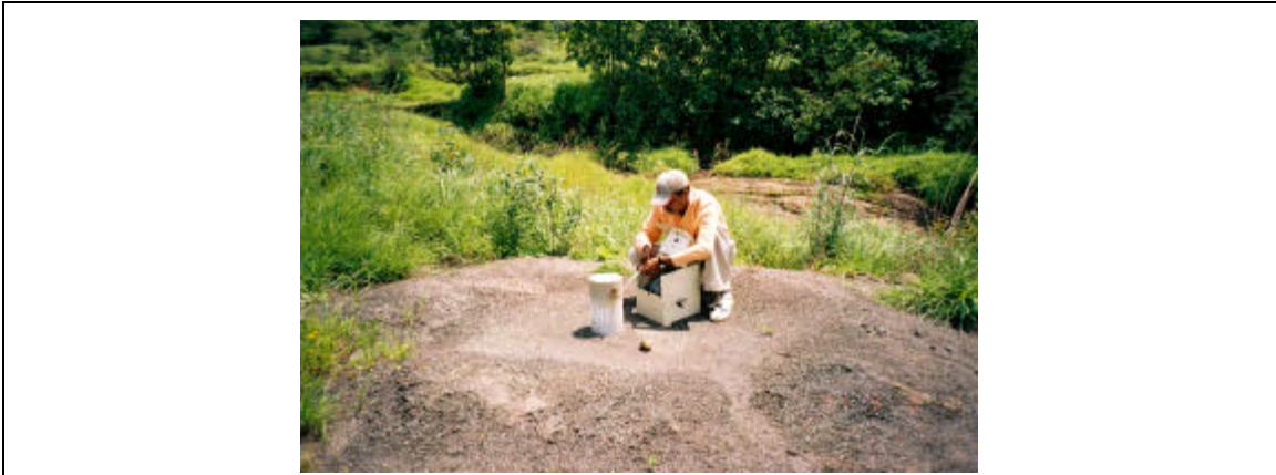
Water level monitoring in boreholes (BH1 here) was done using electronic water level recorders with least count of 0.5 cm.
