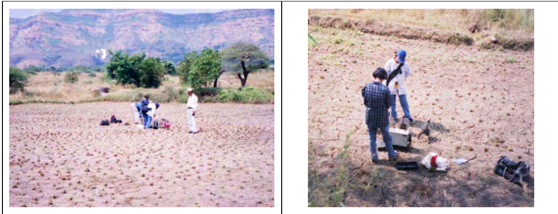
Vertical Electrical Soundings were conducted to determine the lithological layering in the vicinity of CD3, prior to drilling of observation boreholes.
