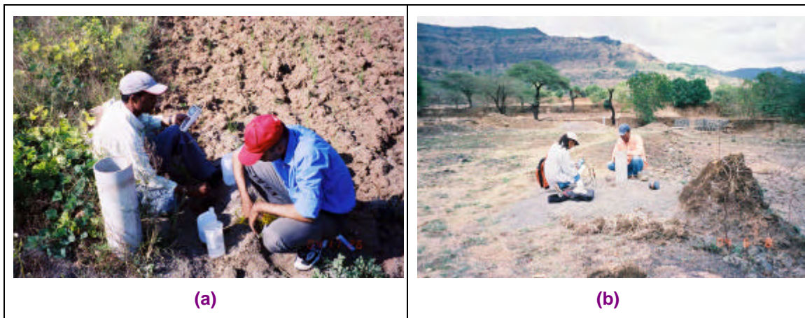
Hydrogeochemical monitoring included collection of water samples from boreholes (a) and other sources like dug wells, river and springs; In situ measurement of field parameters like conductivity and pH were also done (b).
