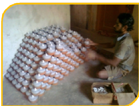
Terafil cakes being manufactured at Modern pottery, Bhubaneswar
