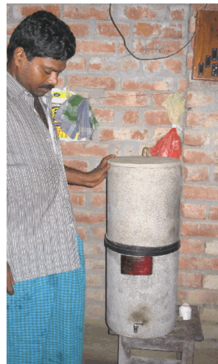
The Nirmal combined arsenic and iron removal filter used in India UNICEF/2003/Keast
