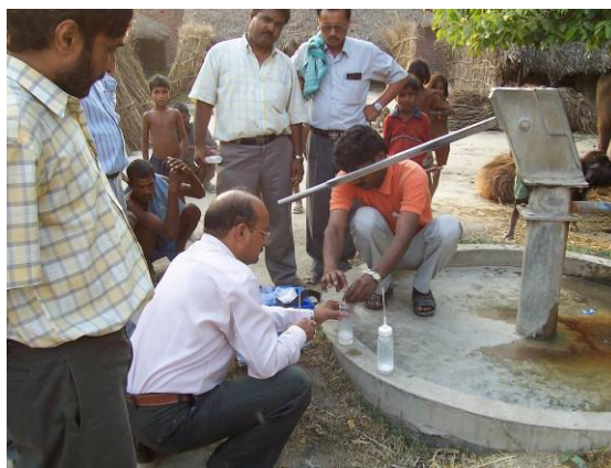
Screening testing using a field test kit in Uttar Pradesh state in India UNICEF/2005/Nickson
