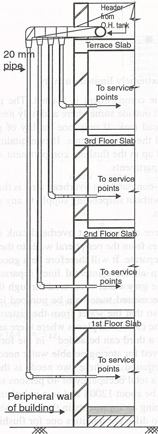
Often, builders give individual pipelines from the overhead tank to each flat in an apartment complex. This is not only expensive but unnecessary. A distribution system that has proved satisfactory in numerous apartment complexes with which the author was involved is illustrated in Sketch 14.6.
