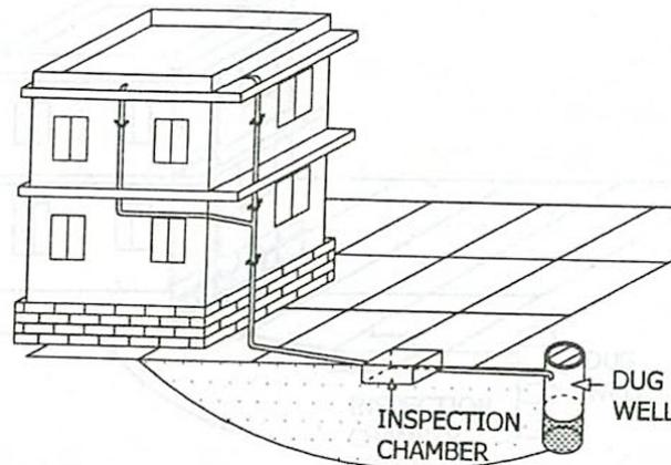
**Picture 7.3** Two downtake pipes (hidden in the photograph) come from the two corners of the cut-out, join together in the small inspection pit. One single pipe from this pit takes the rainwater to the dug well as can be seen in Picture 7.4
